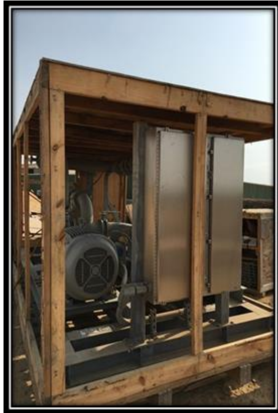
Cooling Water Skid
